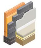
BLOCKWORK 100mm AGLITE Ultima CAVITY INSULATION 100mm Full Fill λ0.032 INTERNAL FINISH Plasterboard on dabs
