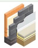
BLOCKWORK 100mm AGLITE Ultima CAVITY INSULATION 75mm Partial Fill PIR λ0.022 with 50mm clear cavity INTERNAL FINISH Plasterboard on dabs
