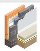
BLOCKWORK 100mm AGLITE Ultima CAVITY INSULATION 50mm Xtratherm X021 with 50mm clear cavity INTERNAL FINISH Plasterboard on dabs
