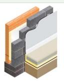
BLOCKWORK 100mm AGLITE Ultima CAVITY INSULATION 75mm Xtratherm CavityTherm INTERNAL FINISH Plasterboard on dabs
