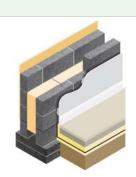
BLOCKWORK 100mm AGLITE Ultima CAVITY INSULATION 125mm Full Fill λ0.032 INTERNAL FINISH Plasterboard on dabs
