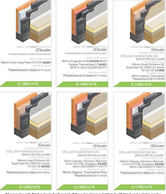
All examples with Brick outer leaf will comply if the outer skin is substituted with block and suitable render
