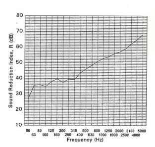
Rating according to BS EN ISO 717-1:1997  $R_w$  (C;C<sub>tr</sub>) = 50 (-1;-4) dB
