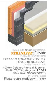
All examples with Brick outer leaf will comply if the outer skin is substituted with block and suitable render
