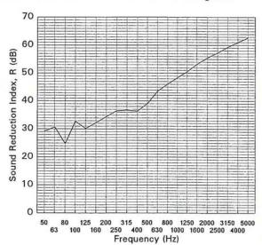
Rating according to BS EN ISO 717-1:1997  $R_w$  (C;C<sub>tr</sub>) = 46 (-2;-5) dB
