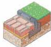
edging with Weathered Kerb
