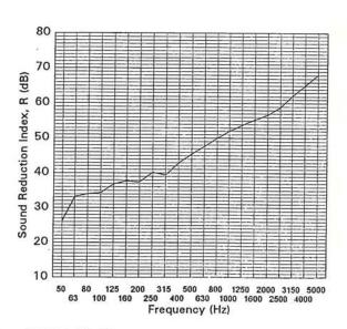
Rating according to BS EN ISO 717-1:1997  $R_w$  (C;C<sub>tr</sub>) = 50 (-1;-5) dB
