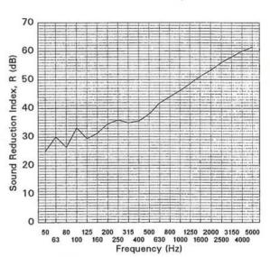
Rating according to BS EN ISO 717-1:1997  $R_w$  (C;C<sub>tr</sub>) = 44 (-1;-4) dB
